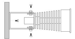
The lamp is attached to the handle with two M4 screws, this allows movement in a vertical
