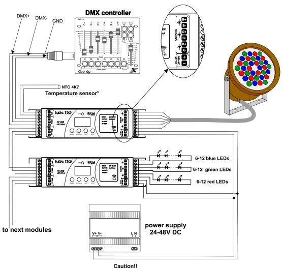
Temperature measurement will be correct only when applying the NTC 4k7 thermistor installed in the lamp.
