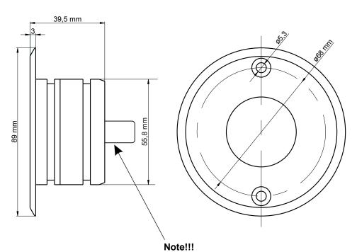
When mounting the lamp, you need to leave enough space for cable gland, from which goes out the power cord.
