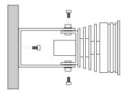
The lamp attaches to the bracket with two M4 screws, this allows movement in a vertical plane.
