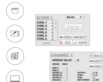
The professional dimmer of AC class, equipped with a colour touchscreen and a LAN interface. The device allows you to control 24 independent channels with a power of 3.6 kW each. The dimmer allows you to control input signals from 6 different sources simultaneously, including:
