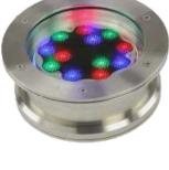
In the PXM offer there are two PxGround lamps designed to be mounted in the ground. The lamps are equipped with the special cover against reflection. The special construction of the housing enables to change the angle of inclination of the LED module inside the lamp, which allows you to direct the light independently (within  $\pm 10^\circ$ ) of the mounted housing.
