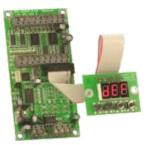
PXM offers 3 devices to convert a DMX signal to the analogue 0-10V signal.
