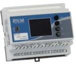
The advanced converter of the DMX signal to DALI and DALI to DMX. In accordance with the DALI standard, up to 64 DALI devices (e.g. ballasts) can be connected to PX255. The device can also convert the control signal in the opposite direction: from the DALI controller to the DMX receiving devices. The menu of the converter allows for any addressing of individual lamps or groups of the devices (maximum 16). In addition, you can define a number of individual parameters for each of the lamps.
