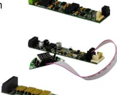
In addition, the offer includes the PX265 MX System driver, which is supplied in the OEM version to allow further building-in to the end user. The driver consists of the modules, which, if properly combined, create the current or voltage driver, or both. The integrated DMX receiver allows you to controll 12 channels.
