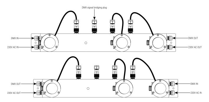
**NOTE!** The user can enter the DMX signal / power supply from any side, please remember that there will be a DMX signal / power output on the opposite side of the lamp.
