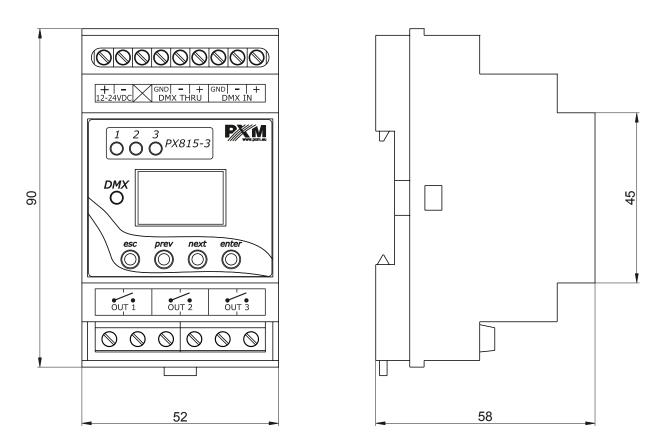
**NOTE!** The layout of the connectors and LED signaling in PX815-2 may differ from the version shown in the technical drawing above (PX815-3).
