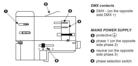
5.2 The cross-section of the DMX GLOBAL Trac<sup>®</sup> Pulse Control
