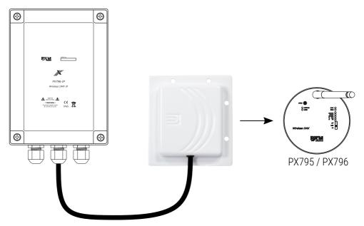
Pairing with a receiver that is not assigned to another transmitter is only possible if the devices are within range. In the transmitter, press the programming key for 0.1 - 1s. Pairing will occur automatically.
