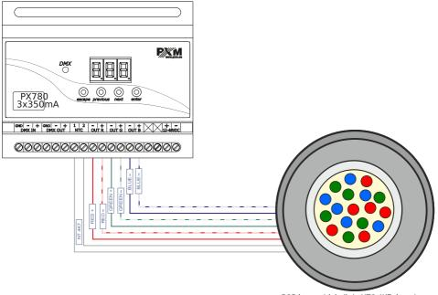
RGB lamp with built-in NTC 4K7 thermistor
