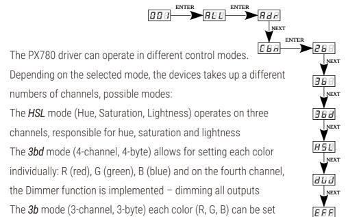
The **2b** mode (2-channel, 2-byte) consists in selecting lightness and one of the 256 colors define by the manufacturer
