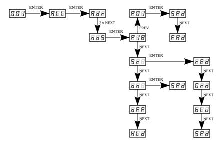
P01 - P18 – choosing a ready program provided in the device software. For each program it is possible to set the speed (SPd) of the effects reproduction on range 0,1 - 99,9s and smoothness of change of steps (FAd) in range 0 - 100, where 0 is a step transition, and 100 completely smooth. Sc –self-programmed scene in which it possible to set values for RGB colors (FEd, GFD, FED) in range FED0 after decay DMX signal in range FED1.
