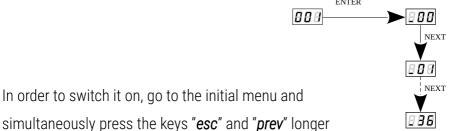
The message BBB will appear in the screen, which means that none of the channels is controlled in 100%. Next, enter the selected channel (with the keys "next" and "prev"). Next channels will be switched on for 100%. In order to
