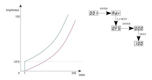
This parameter is useful when the diodes connected to the driver show unstable functioning at the low control levels. In such a case the increase in the value *OFFSET* can result in achieving better dimming effects.
