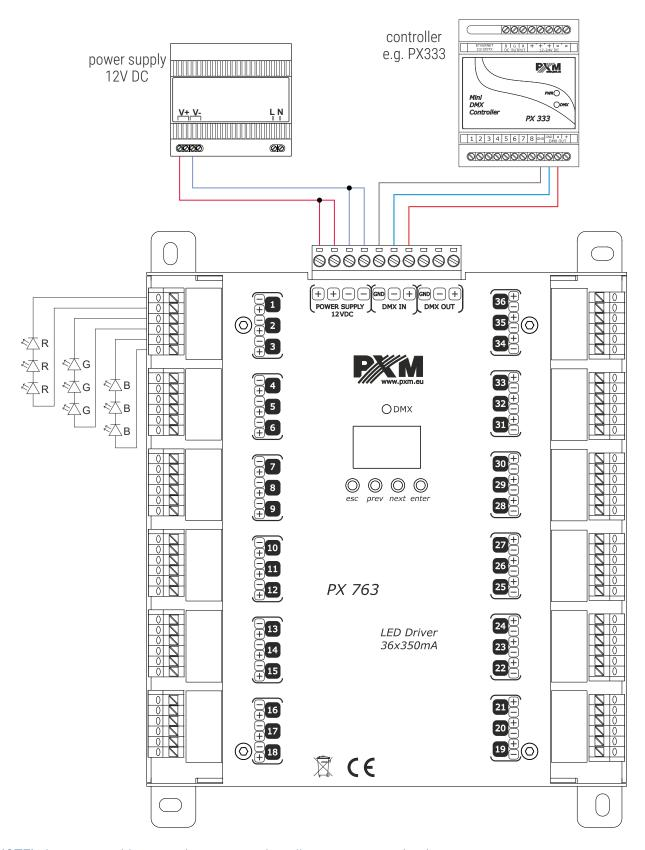
**NOTE!** The power cables must be connected to all connectors on the device.
