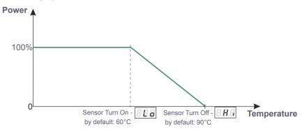
If this function is activated and the temperature sensor is incorrectly connected or there is no sensor, the driver displays a relevant message – *Er0* at the current temperature location, and instead of the first DMX address, i.e. at the very beginning of the menu. To disable the message, connect an appropriate sensor or disable the temperature limit.
