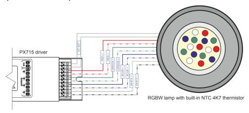
The connection of the NTC 4K7 thermistor is applicable only when one lamp is connected to the driver. This is due to the fact that the device can read the temperature from only one lamp.
