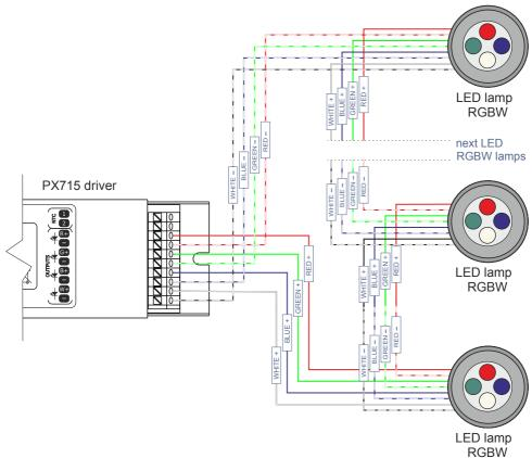
Example connection the PX715 driver to the LED RGBW lamp:
