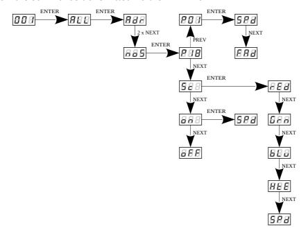
P01 - P18 – choosing a ready program provided in the device software. For each program it is possible to set the speed (SPd) of the effects reproduction on range 0,1 - 99,9s and smoothness of change of steps (FAd) in range 0 - 100, where 0 is a step transition, and 100 completely smooth.
