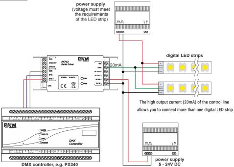
Connecting power from one shared source to the digital LED strip and to the driver
