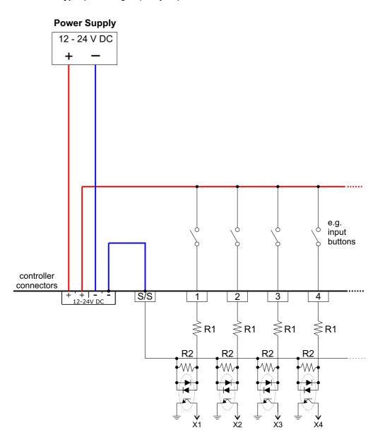
• Source in type - negative logic input - "joint mass"
