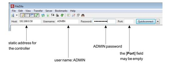
The connection to the controller via FTP can be useful when it is not possible to upload the firmware update via the application. Then, replace the "UPGRADE.UPG" file in the controller and exit the core mode (by force). The controller will be automatically updated.
