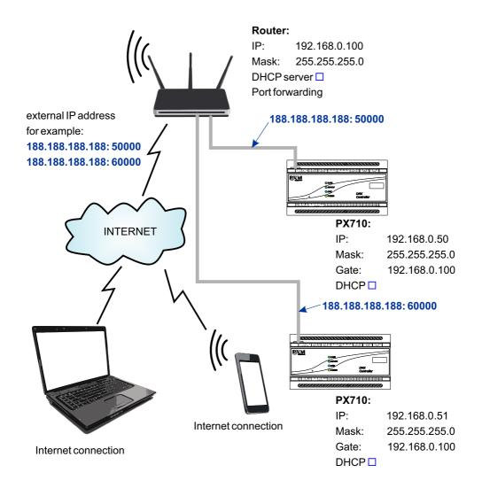
Then, to connect to the controller via the Internet, in the application window "Connect to device" in the "Address" field enter the IP address of the router (assigned by your ISP), which in this case is 188.188.188, and in the "port" field enter the lower of the forwarded ports for the first controller, in this case port 50000. To connect to the second controller, change the port to the lower one of the ports forwarded to the second controller (in the example: 60000).
