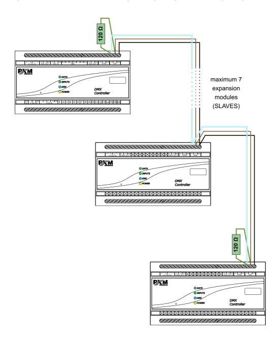
**NOTE:** It is necessary to connect a 120  $\Omega$  terminating resistor to the first and last device.
