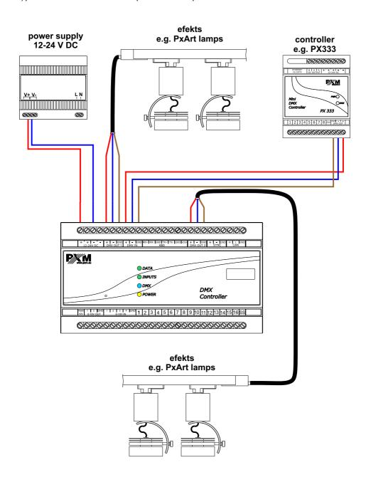
b) Connection between a master controller (MASTER) and expansion modules (SLAVE)
