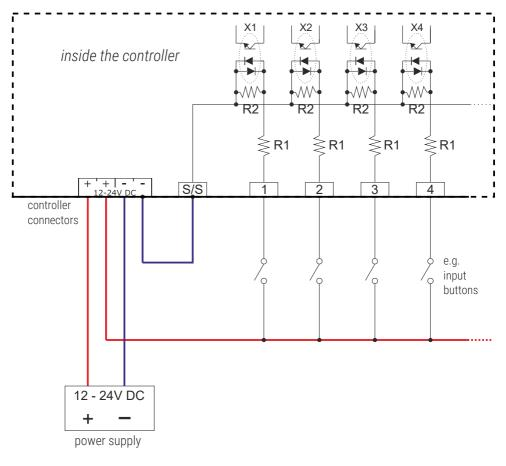
e) connection of digital inputs (source in) - negative logic input - "joint mass"
