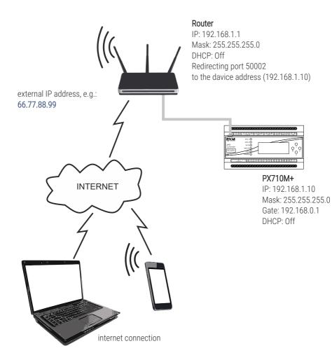
**NOTE!** If there are two controllers in network, the first one should be forwarded to the port 50002 and the second to e.g 60002 (the destination port is always port 50002).
