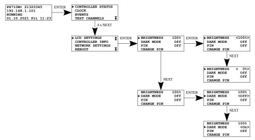
NOTE! Active DARK MODE turns off the backlight only on the main window.
