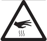
While working outdoors in normal conditions, the housing unit can heat up to +65°C. Make sure that accidental contact with the device during use is impossible.
