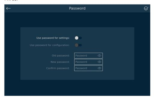
To protect the settings with a password, slide the switch *Use password*, enter the current password. The default password for devices with a system version below 1.0.38 is "admin", for newer versions it is the serial number of the device. Then enter the new password twice. Selecting the *Use password for configuration* option will block the selection of configuration in the main window – entering a password will be required.
