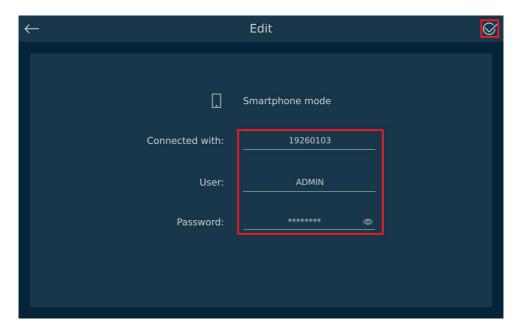
After entering the login details for the controller, press the save changes button  $\bigotimes$  located in the upper right corner of the screen.
