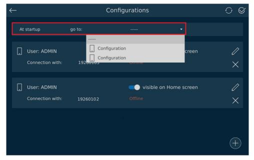
**NOTE!** All changes made must be saved using the button  $\bigcirc$  located in the upper right corner of the screen.
