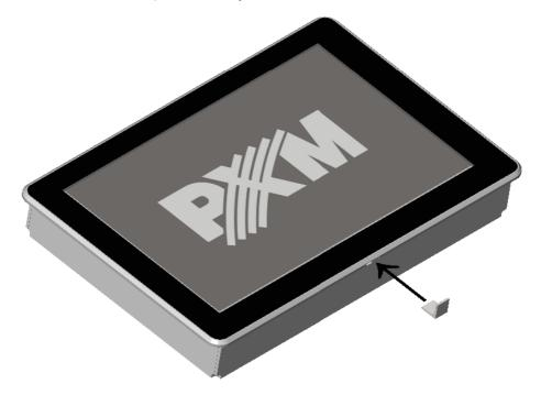
When the metal angle is inserted under the screen and pressed down, swing the bottom of the screen down and pull it towards you.
