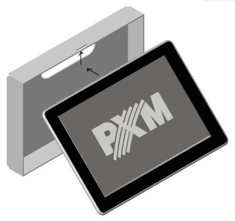
Then, paying attention to the fact that the tooth is in the hole, press the bottom of the screen towards the metal housing until you hear a characteristic click.
