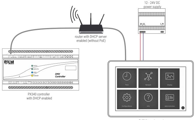
PX703 touch panel with DHCP enabled (power from an external power supply)
