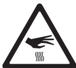
**While working at an ambient temperature of 25°C housing unit can heat up to 90°C. Because of the danger of burns, avoid direct contact with the casing.**
