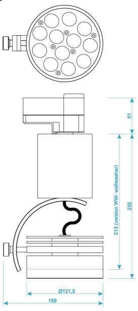
Dimensions are given in millimetres
