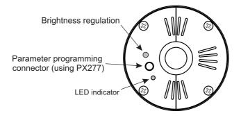
The programming button above the reflector has been equipped with a diode which indicates the condition of the lamp. Depending on a situation, the diode signals the following:
