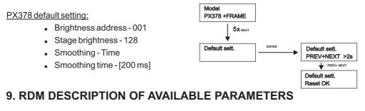
PX378 supports the DMX-RDM protocol. DMX protocol in its assumption enables one-way data flow while its extension, the RDM protocol, can transmit information in two ways. This makes the simultaneous receiving and sending of information possible and allows for monitoring the operation of devices compatible with the RDM protocol as well as possibly changing the configuration of their parameters.
