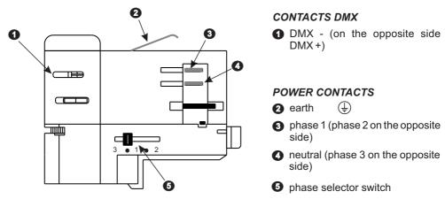
5.2. Section through the DMX GLOBAL Trac Pulse control current rails.
