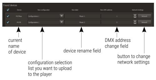
To search for devices in a local network in the **[Devices]** menu select the **[Search]** command. All devices found are displayed in the device list. **[Set background]** – an image that is displayed when no file is uploaded. The default background color is black, but any different image in the \*.jpg format can be uploaded.
