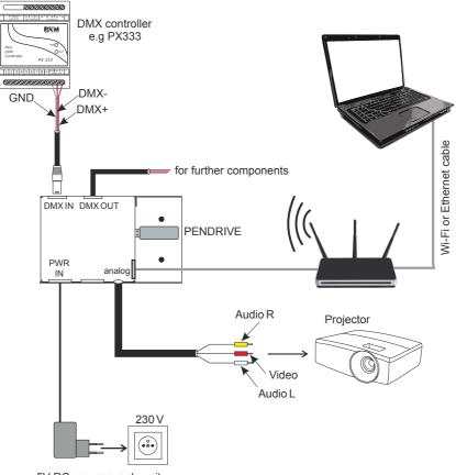
5V DC power supply unit included with the device
