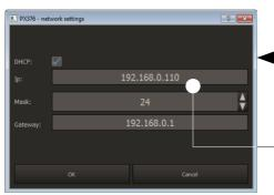
if the function is selected, address will be automatically assigned from a DHCP server, if not – a static address will be used
