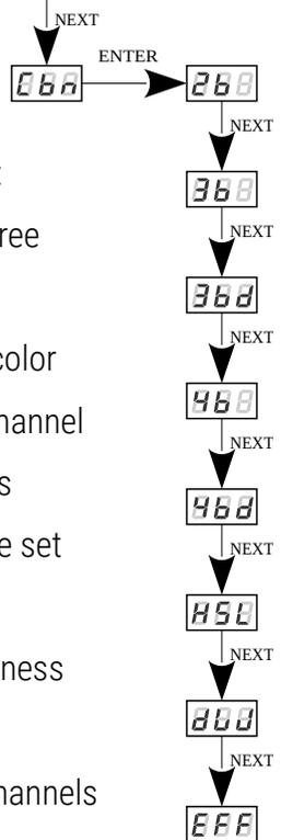
The **EFF** mode – effects control – it is available on 8 DMX channels and allows to choose the right effect and parameters (description of the **EFF** mode is on the next page):
