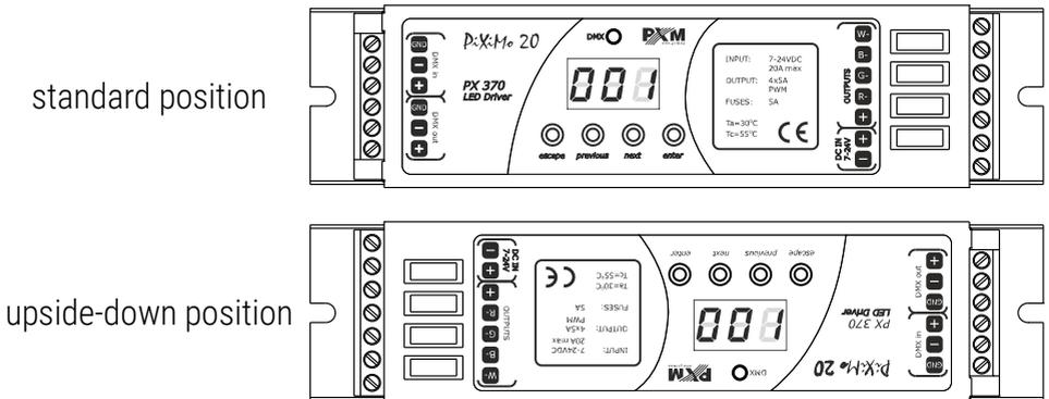
**NOTE!** The keys on the reverse of the display are set in the same way as the normal position, keys are reversed.
