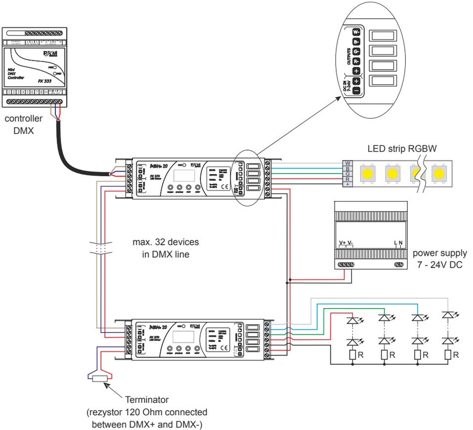
**NOTE!** That the driver is common anode type device. It is possible to connect lamps with 5-wires cable with a common "+" only.
