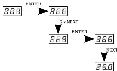
**NOTE!** In the *L0* version, the frequency setting is in the range of 488Hz – 25kHz. Information whether the device is the *L0* version is displayed during device start-up.
