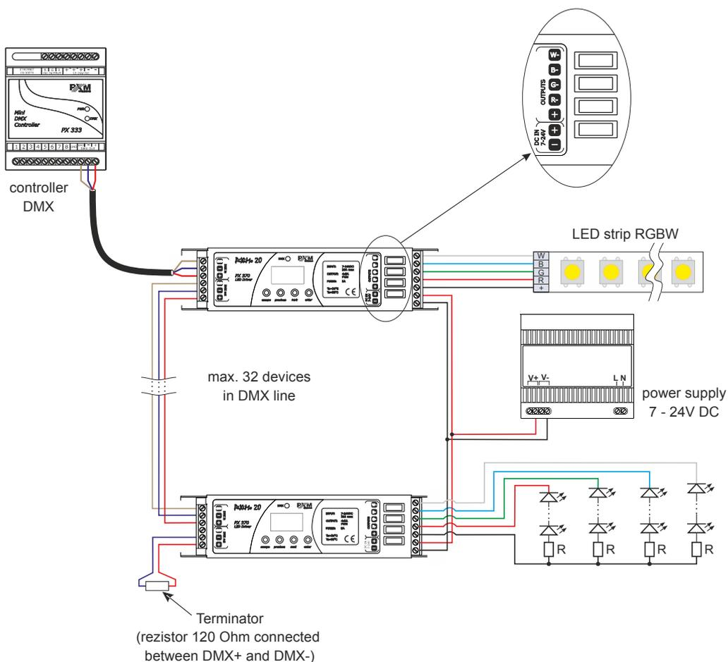
**Note!** The driver is common anode type device. It is possible to connect lamps with 5-wires cable with a common "+" only.
