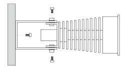
The lamp is attached to the holder with two M4 Allen screws and can be rotated
