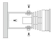
The lamp is attached to the holder with two M4 Allen screws and can be rotated vertically. The handle is attached to the ground with one M5 screw, which in turn allows for rotation in the horizontal plane.
