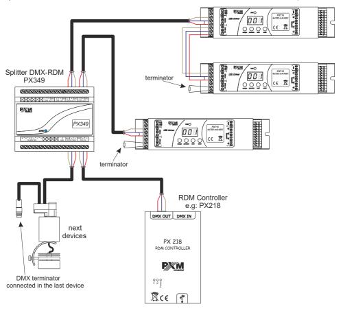
b) shorting of 120R pins – if the splitter is the last device and no receiver is connected to the *DMX THRU* output, the bridge on these pins acts as a terminator
