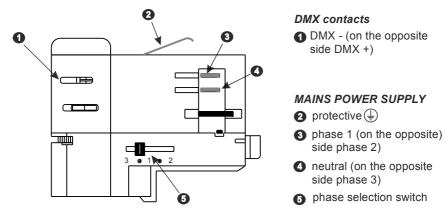
7.2 The cross-section of the DMX GLOBAL Trac<sup>®</sup> Pulse Control
