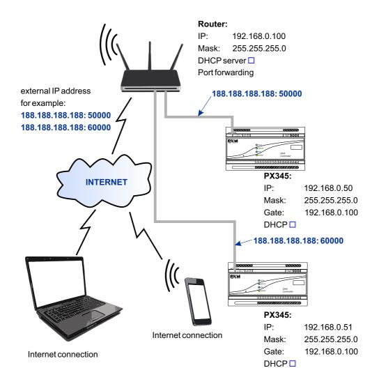
Then, to connect to the controller via the Internet, in the application window "Connect to device" in the "Address" field enter the IP address of the router (assigned by your ISP), which in this case is 188.188.188.188, and in the "port" field enter the lower of the forwarded ports for the first controller, in this case port 50000. To connect to the second controller, change the port to the lower one of the ports forwarded to the second controller (in the example: 60000).
