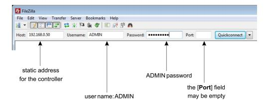
The connection to the controller via FTP can be useful when it is not possible to upload the firmware update via the application. Then, replace the "UPGRADE.UPG" file in the controller and exit the core mode (by force). The controller will be automatically updated. Using the FTP you can also delete the preloaded configuration.
