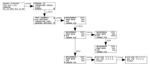
**NOTE!** After activating the function of securing the device with a PIN code, it is recommended to change the PIN from the default one to the one defined by the user.
