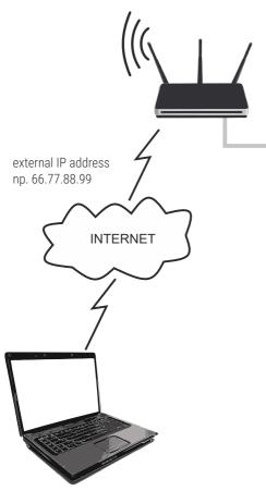
Router IP: 192.168.1.1 Mask: 255.255.255.0 DHCP: Off Redirecting port 50000 and 50001 to the device address (192.168.1.10)
