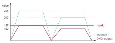
• **maximal** – it converts all the values in the channel that are greater than the value of the mask to the value of the mask
