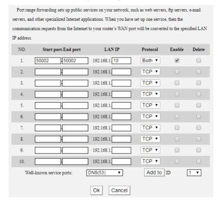
If there is no option to set one port forwarding in the router, create a range (from 50002 to 50002). If everything is correctly configured to connect to the controller from the (external) internet network, select the *Remote login* in the application (PxMini or PxMobile), and then enter the *User* and *Password* of the user and *Host* (assigned by the internet provider, in this case 66.77.88.99), in the *Port* field enter the port number (50002).
