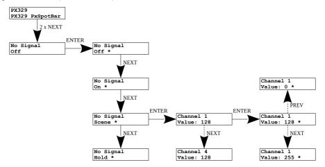
An additional parameter is **[No Signal Time]**, which defines the entry time of the selected option in the **[No Signal]** menu. This parameter is set in the range of 1 to 10 seconds.
