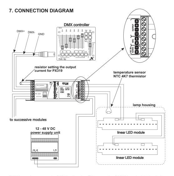
PX319 must be connected to DMX line in series. This means that DMX IN terminals in the device must be provided with the driving cable, and then from DMX OUT connector the driving cable must be provided to other DMX receivers.
