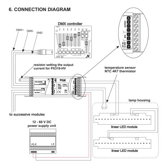
PX319-HV must be connected to DMX line in series. This means that DMX IN terminals in the device must be provided with the driving cable, and then from DMX OUT connector the driving cable must be provided to other DMX receivers.
