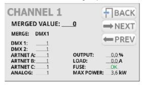
The device has a built-in merger system with an option to select one of 13 priorities, including permanent activation of any circuit, regardless of the controls. The advanced electronics allows to address each output channel in any way, to select and edit the driving characteristics (5 factory characteristics, 5 user's characteristics), and to set limits for voltage and output current for each channel individually.
