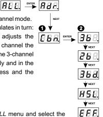
To set the colours mode, enter the *Cbn* feature in the *ALL* menu and select the required colours mode: 2b for 2-byte mode, 3b for 3-byte mode, 3bd for RGBDimmer mode or HSL for Hue/Saturation/Lightness. There is also EFF mode-description on next site.
