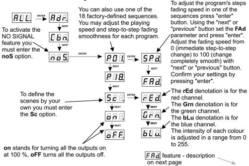
Feature FBB. - to adjust the program's steps fading speed in one of the sequences press "enter" button. Using the "next" or "previous" button set the FAd parameter and press "enter".
