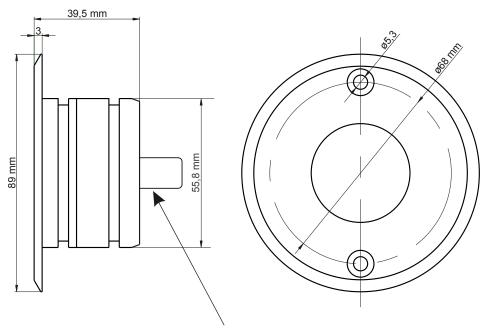
When mounting the lamp, you need to leave enought space for cable gland, from which goes out the power cord
