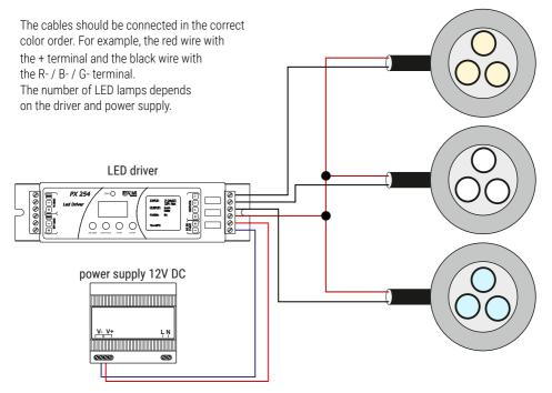
b) diagram of connecting the lamp with voltage power supply
