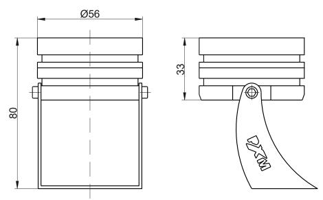
**NOTE!** When mounting the lamp, you need to leave enough space for cable gland, from which goes out the power cord.
