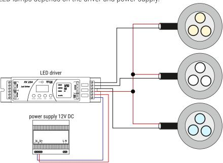
Example of connecting PX284 lamps to the PX254 driver with an option of a 0.5 m cable with a Weipu SP13 3 PIN connector.
