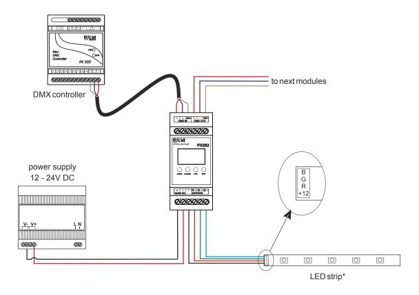
\* typical LED strips are supplied with 12V DC – then the PX282 has to be connected also the 12V DC power supply with adequate power, in the case of using LED strips supplied with 24V DC, the PX282 has to be connected to 24V DC power supply that power is matched to the length of the strip.
