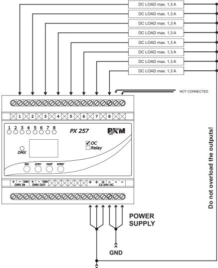
**NOTE**: To evenly load each of power supply dedicated pins connect power supply conductors (12 - 24V DC and GND one) to all suitable PX257 pins - according to diagram.
