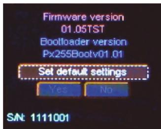
To restore default setting press *enter* button, then select the *Yes* button and again approve with *enter*. In the case of incorrect choosing option, you can go back by selecting *No*, or go directly level up in menu by pressing *escape*.
