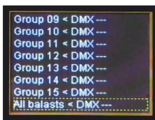
**NOTE!** Patching from DMX signal to DALI, e.g. channel 1 to ballast 0 is shown as **Balast 00 < DMX 001**.
