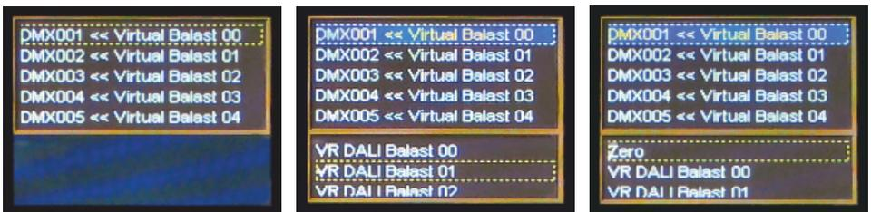
**NOTE!** Patching from DALI signal to DMX, e.g. virtual ballast 0 to DMX address 1 is shown as **DMX 001 <<< Virtual Ballast 00**.
