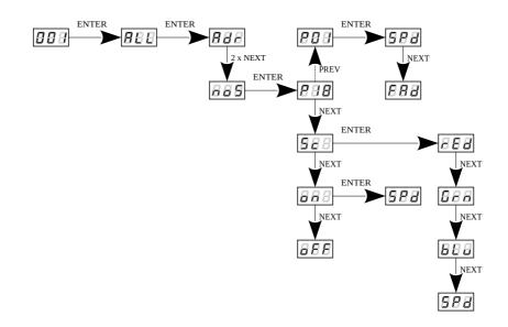
P01 – P18 – choosing a ready program provided in the device software. For each program it is possible to set the speed (SPd) of the effects reproduction on range 0,1 – 99,9s and smoothness of change of steps (FAd) in range 0 – 100, where 0 is a step transition, and 100 completely smooth.
