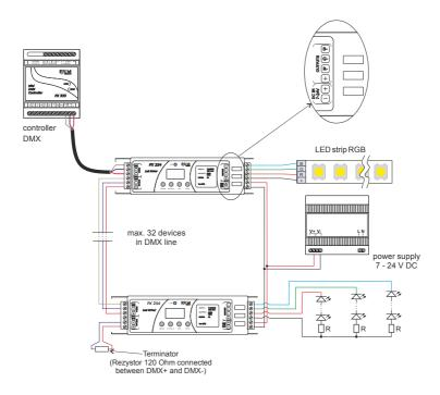
Please note that the driver is common anode type device. It is possible to connect lamps with 4-wires cable with a common + only.
