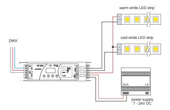
With such a connection of strips, in dW control mode, the value 0 on the color temperature channel corresponds to warm white color, and value 255 – cold white
