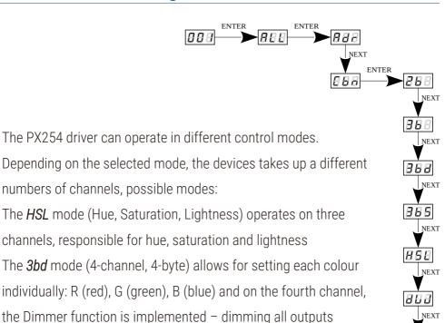
The *3bS* mode(3 RGB channels + Shutter) 6-channel mode allows
