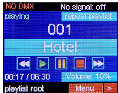
The start menu screen if the DMX signal is received
